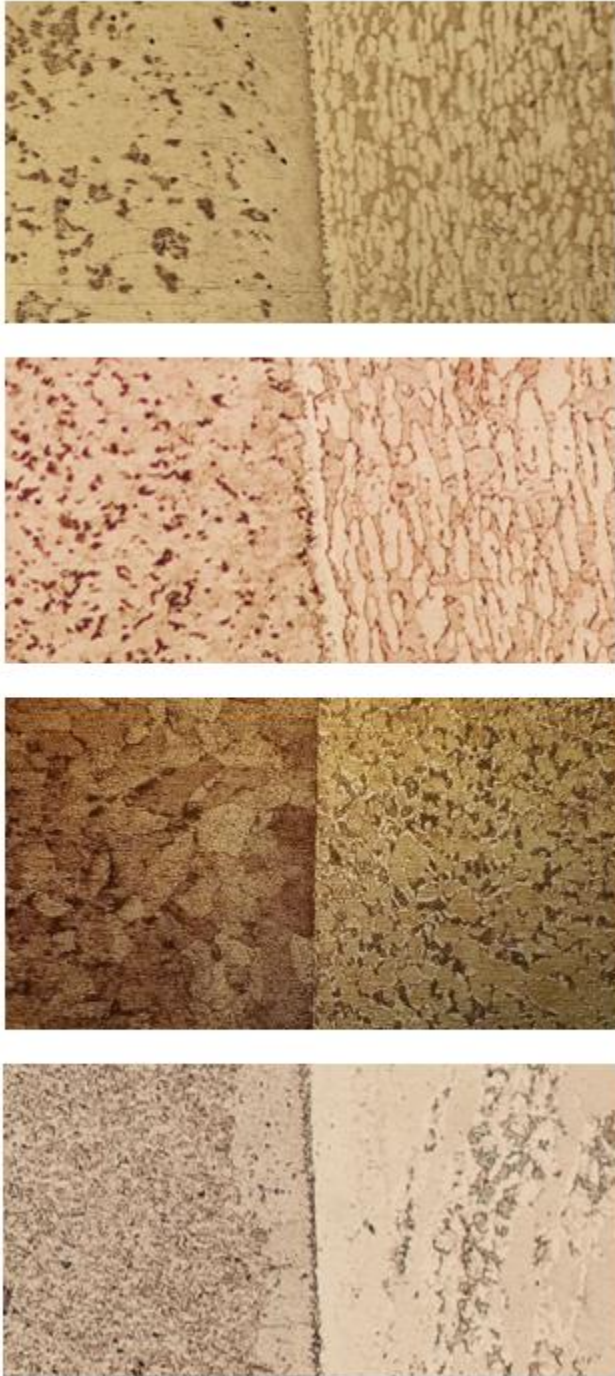
Figure 4: Microstructures of welded joints at 1150°C: (a): 45 min, (b): 120 min, (c): 300 min, and (d): 1200 min.
